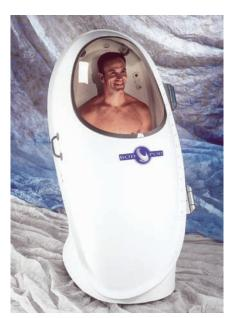
**FIGURE 8-5** A pod for measuring body composition. The BOD POD uses air displacement technology to measure body composition. (Courtesy Life Measurement, Inc, Concord, Calif.)
